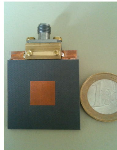
Fig. 6 Photo of the fabricated prototype of ACMPA
